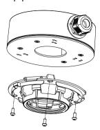
Make the proper connections to the cable harness and conceal the cables. Reattach the camera body to the base and adjust the position of the lens.
