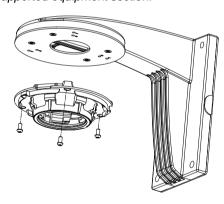
3. Make the proper connections to camera harness and conceal the cables. Reattach the camera body to the base and adjust the position of the lens.
