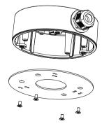
Remove the camera body from the turret camera base. Attach the base to the turret adapter plate by inserting the B screws into holes 2 or B screws into holes 1. Refer to the *Supported equipment* section.
