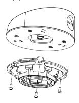
Make the proper connections to the camera harness and conceal the cables. Reattach the camera body to the base and adjust the position of the lens.
