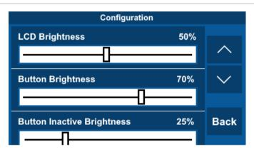
Use the Enter # key and \* Menu key or the Up and Down arrows to navigate the list. The configuration options are described in the following sections.
