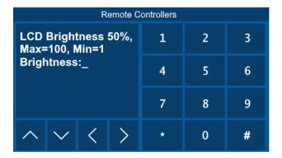
Press the buttons that correspond to the desired value from 1% to 100% levels, and then press the # button (or press Enter # key) to apply the new value.
