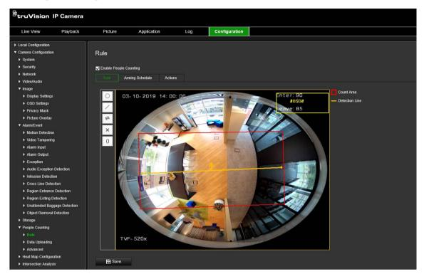
1) Click / to draw a detection line. An orange detection line will appear on the image.
